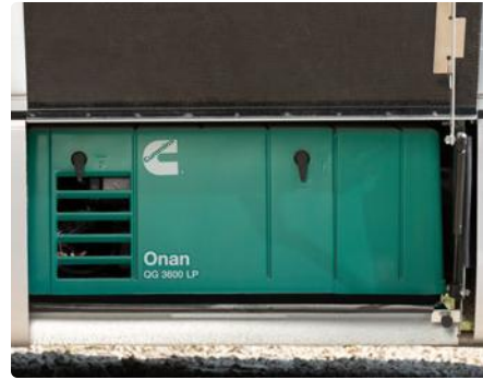
3.6 kW LP Generator Auto Start and Auto Changeover Switch
